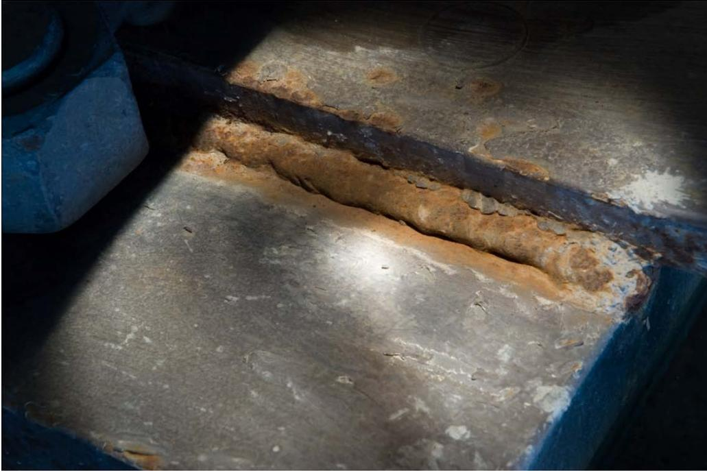
Unacceptable weld (overlap at the bottom toe, undercut at the top toe, inadequate cleaning)
